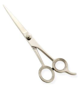
Professional Razor Edge Barber Scissor Movable Screw, Fixed Finger Rest. Available Sizes. 4 in, 4.5 in Details. Razor edge hair dressing scissors made of Japanese stainless steel J/2 - 420, HRC° (hardness) 52° - 55°. Also Avaiable in 440c, HRC° (hardness) 60° - 65°. Available in Fix, Limitaion, Adjustable and hand adjustable screws with and without leaf spring.
