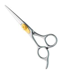
Hand-made two piece style. Japanese steel with HRC 50-55 hardness. Hollow-ground blades. Removable Trumpet finger rest. Available Sizes: 4.5",5.0",5.5",6.0",6.5",7.0"
